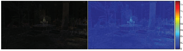
Fig. 20. Our result differs from the reference MC, as shown by these difference and intensity images (showing the norm of the error) for the scene in Fig. 19. The differences occur in regions of high-frequency detail that our bilateral filter tries to preserve but ends up slightly overblurring due to the significant amount of noise in the input image. The transparent vase on the table also exhibits differences because the path tracer does not have enough rays at 8 samples/pixel to compute the inter-reflections inside the glass.
